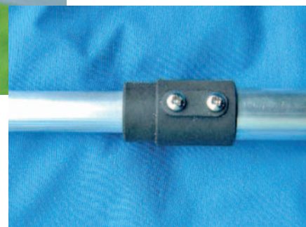
● Fig. 4 (left): The Gamma match rod attaches to a moulded SO239 socket, making construction easier and no soldering is needed.
